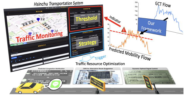
Figure 8: Integrating our framework with the city’s transportation system, by utilizing GCT flow for predictive mobility insights, activates a threshold-based alert system for optimal traffic management. This achieves practical convergence of telecom data and transportation needs through driver notifications, CMS for alternative routing, and optimized traffic signal control.
