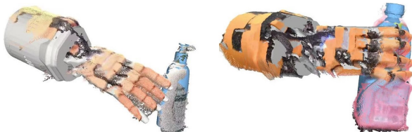
Figure 3: Visualization for well-aligned dexterous hand's mesh (white), object's mesh (blue), and the colored point cloud of the scene, demonstrating that the calibration and synchronization between robot and camera is accurate and the 6D pose estimation for object is also precise.
