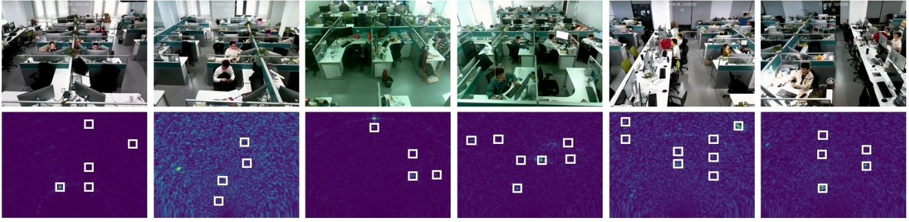
Figure 4: Data samples of our collected RF-UNIT dataset. The first row demonstrates the RGB images of six office scenarios. The second row illustrates corresponding RF heatmaps and tracking annotations. Each frame spans a spatial region of 9m \times 10m . Our dataset consists of different number of individuals and obstacles leading to severe interference.
