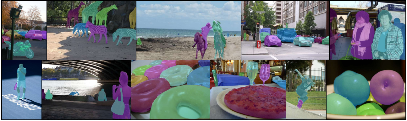
Figure 5: Qualitative results of MISA with ResNet-101 backbone and SOLOv2 framework on COCO val dataset. The model demonstrates commendable performance in object segmentation without any mask supervision.
