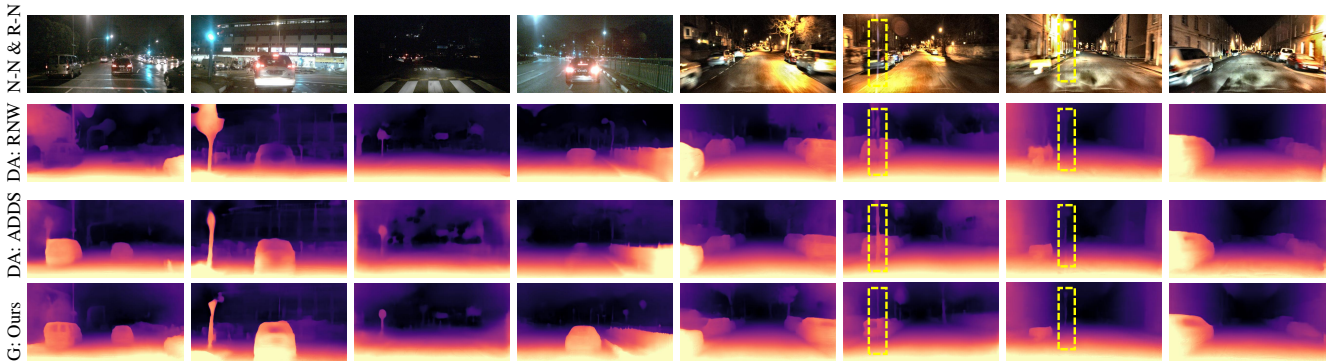
Figure 5: Qualitative results on nuScenes-Night (First four columns) and RobotCar-Night (Last four columns). We leave more visual comparisons to the supplementary material . Compare to DA types methods, our training applies no images from the nuScenes or Oxford RobotCar datasets.
