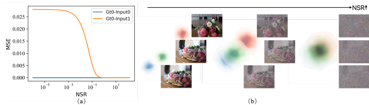
Figure 2: Progressive noise addition to images. (a) Relationship between MSE and NSR of noisy images, for the same image pair (blue curve) and different pairs (orange curve). (b) Data distribution at various NSR ( 10^{-6} , 10^{0.4} , 10^{1.8} ), where blue and green contour plots are for the corresponding large-aperture and small-aperture images, respectively, and red contour plot is for another image. As the noise level increases, the distinctions between images (and data distributions) gradually diminish, eventually converging towards standard Gaussian noise. This suggests that initiating sampling with standard Gaussian noise fails to leverage any prior information.
