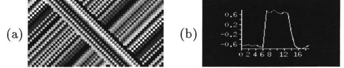
Figure 8: One-dimensional motion. (a) Stimulus I(x, t) - a one-dimensional surface is moving to the right in front of a background moving to the left; (b) Spatiotemporal orientation recovered for the stimulus for a given instant in time. Leftward vs. rightward motion is successfully extracted.
