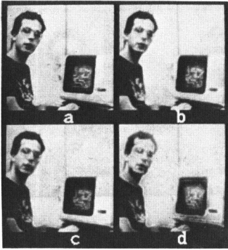
Figure 2: Compression using the Laplacian pyramid. a) Four quantization steps at all levels (2.66 bits/pixel). Two steps at the lowest level, four steps at all other levels (1.66 bits/pixel). c) Two steps at the lowest level, eight at all other levels ( 2 bits/pixel). d) Two steps at all levels (1.33 bits/pixel).
