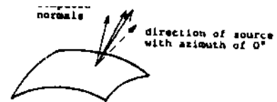
Figure 1b. Computed normals at a single point with source at 0 exhibiting specularity. Intensity value from this source is elevated causing a high deviation among these normals.
